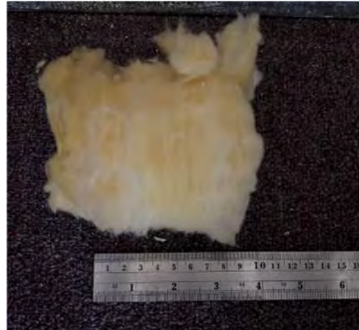
Figure 11 - 3.5" Batt insulation in Manager Office
